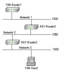
TAR-Router1: Applicant (if router) or Vendor C/D Router TAR-Host1: Applicant (if host) or Vendor A/B Host TAR-Host1: Applicant (if host) or Vendor A/B Host REF-Router2: any router REF-Router3: any router
