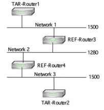
TAR-Router1: Applicant Implementation TAR-Router2: Vendor C/D Router REF-Router3: any router REF-Router4: any router
